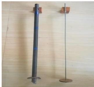
Fig. 2. Helical anchor and anchor plate with rod.
