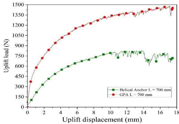
Figure 6. Uplift load-displacement behavior of Helical anchor and GPA at L = 700 mm
