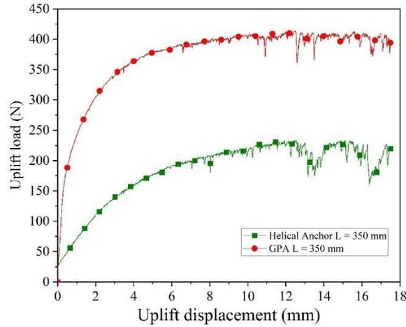
Figure 4. Uplift load-displacement behavior of Helical anchor and GPA at L = 350 mm
