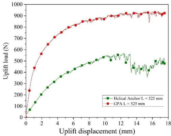
Figure 5. Uplift load-displacement behavior of Helical anchor and GPA at L = 525 mm
