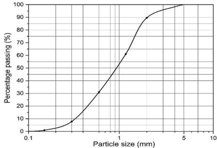
Fig. 1. Particle size distribution curve of sand.
