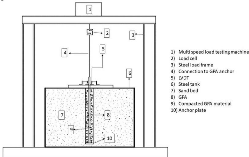
Fig. 3. Schematic diagram of uplift test apparatus
