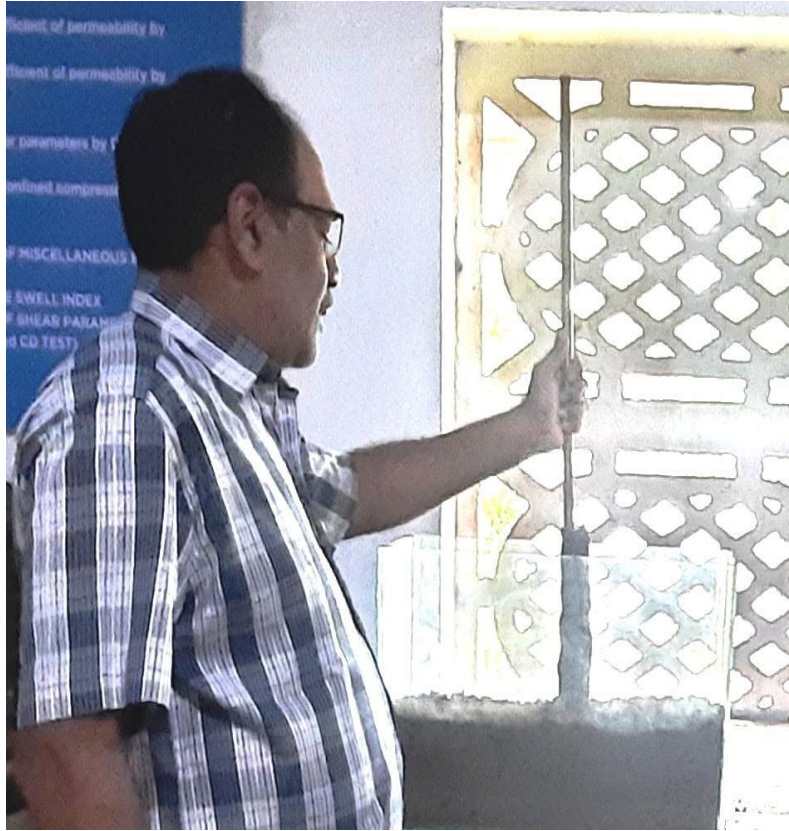
Fig 2.0. Model box with soft clay bed installed with treated jute fibre encased stone columns.
