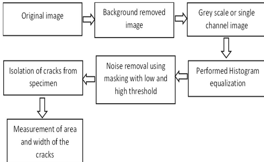
Fig. 3. Schematic diagram of quantification of cracks generated using MATLAB digital image processing.
