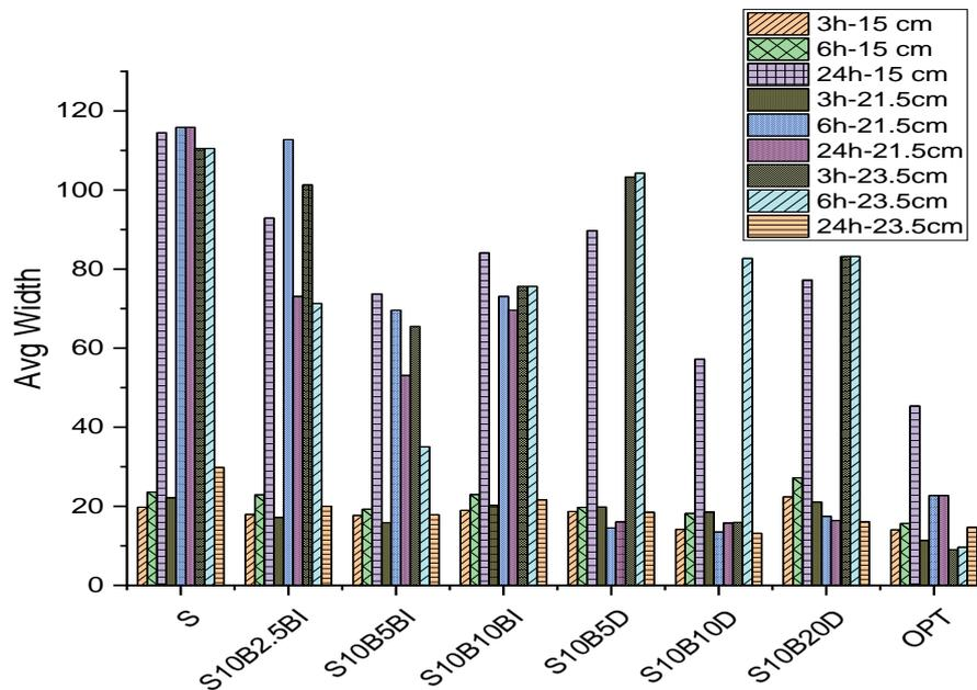
Fig. 8. Variation of average width of cracks for the compositions.
