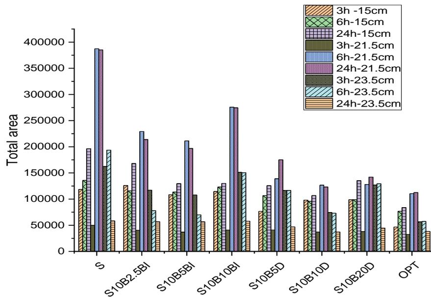
Fig. 5. Variation of total area of cracks for the compositions.
