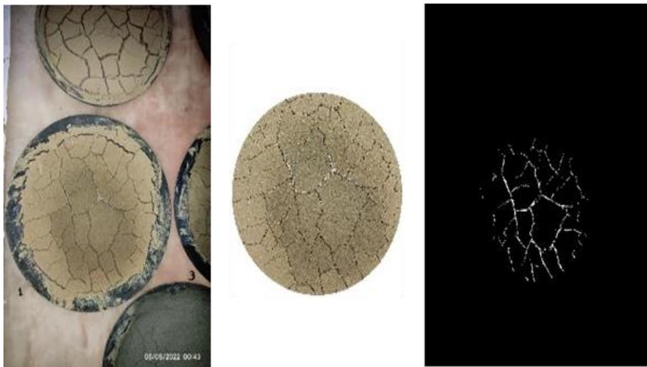
**Fig. 2.** Background removal and quantification of cracks using MATLAB digital image processing.
