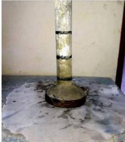
Fig.1 bell-shaped anchor with geo-textile tie
