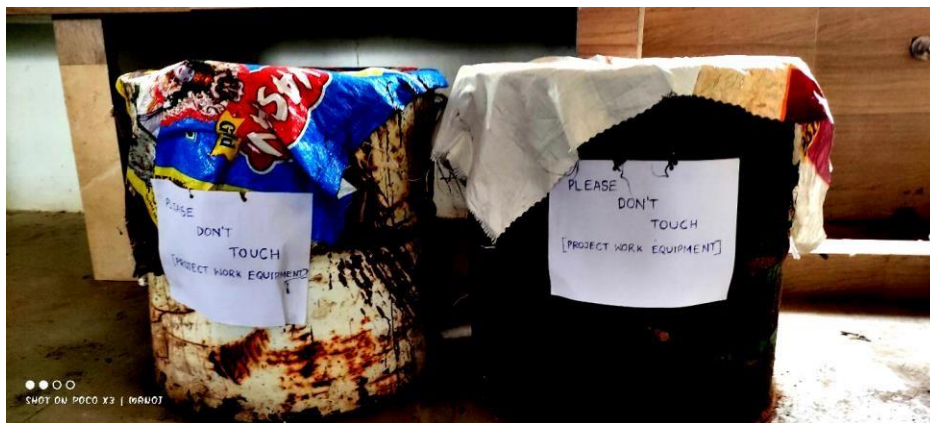
Fig 3.5: Soil with lime columns in Tank1 and soil with flyash-lime columns in Tank 2 are placed for Curing
