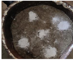
Fig 3.3: Surface of soil block after lime piles installation.
