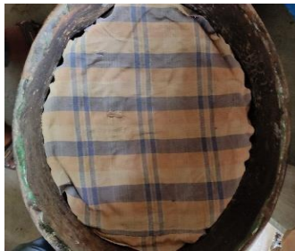
Fig 3.4 a: Cloth covering soil block.
