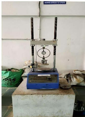
Fig. 3. Unconfined compression test setup.
