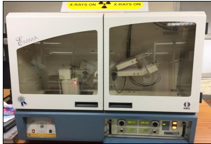
Fig. 5. Mineralogy study with XRD.
