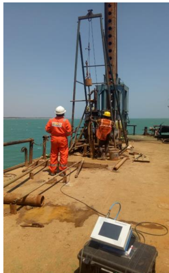
Fig.5. SPT Energy measurements at Site-B
