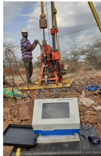
Fig.6. SPT Energy measurements at Site-C
