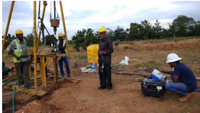
Fig.4. SPT Energy measurements at Site-A.
