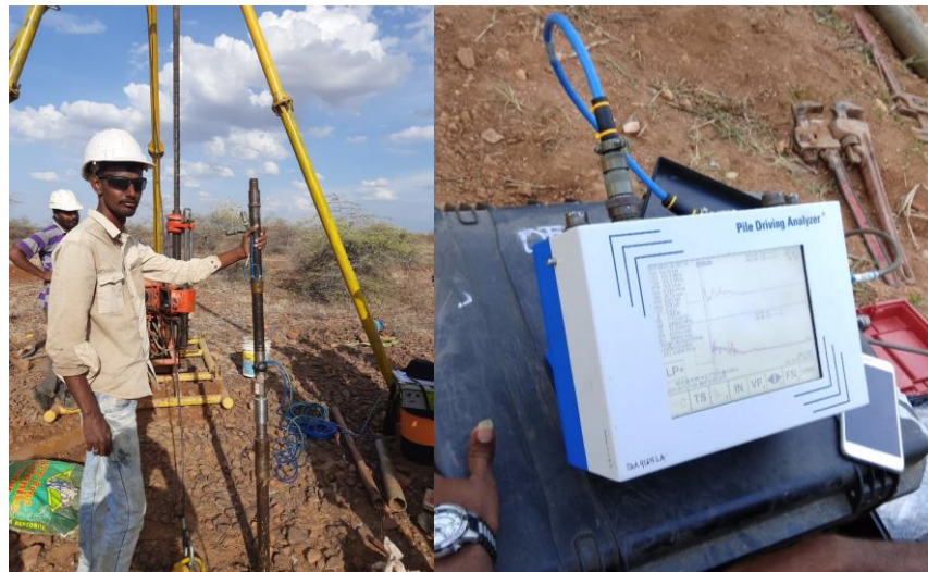
Fig. 3. a) Instrumented Rod b) Pile Driving Analyser for Energy Measurement
