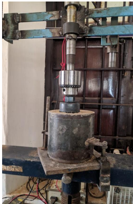
Fig. 1. Laboratory drilling test set up
