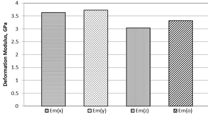
Fig. 2. Anisotropy in deformation modulus at applied stress 10 MPa
