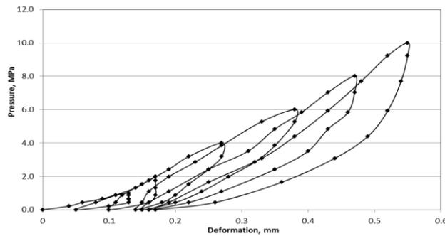
**Fig. 7.** Stress-deformation plot for GJT
