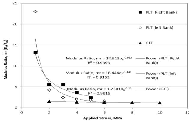
**Fig. 6.** Modulus ratio vs applied stress curve
