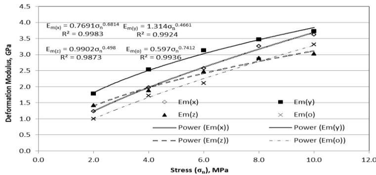
Fig. 3. Variation in deformation modulus with variation in stress
