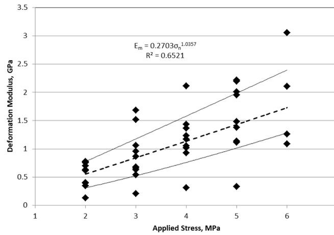
**Fig. 4.** Variation of deformation modulus by PLT
