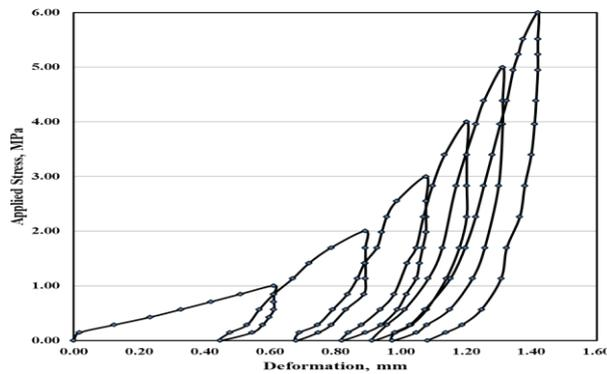
**Fig. 8.** Stress-deformation plot for PLT
