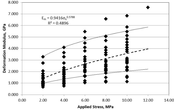
**Fig. 5.** Variation of deformation modulus by GJT
