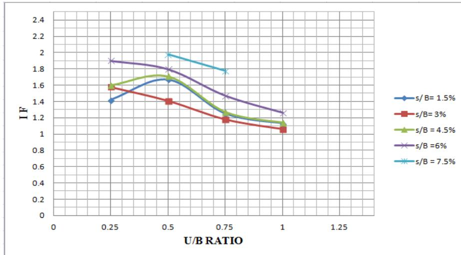
**Fig.11.** Improvement factor vs u/B ratio for various s/B ratio
