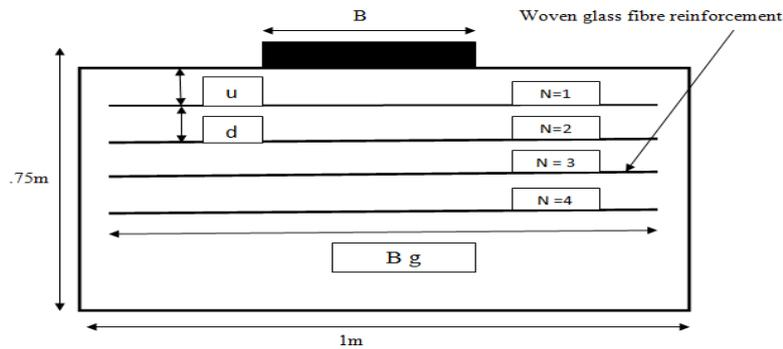
**Fig.4.** The layout of WGF reinforcement
