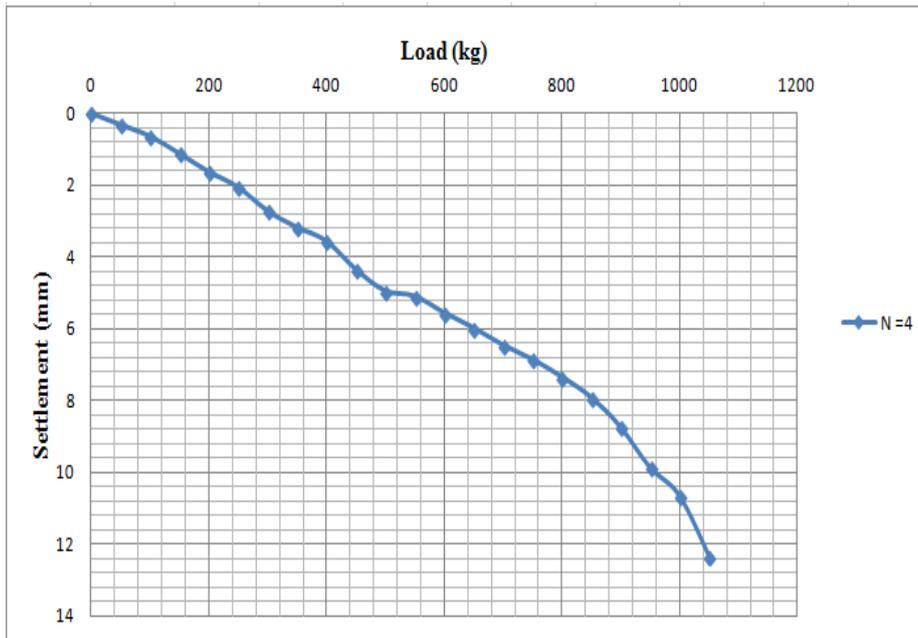
Fig.14. Load vs settlement curve for four layers of WGF reinforcement
