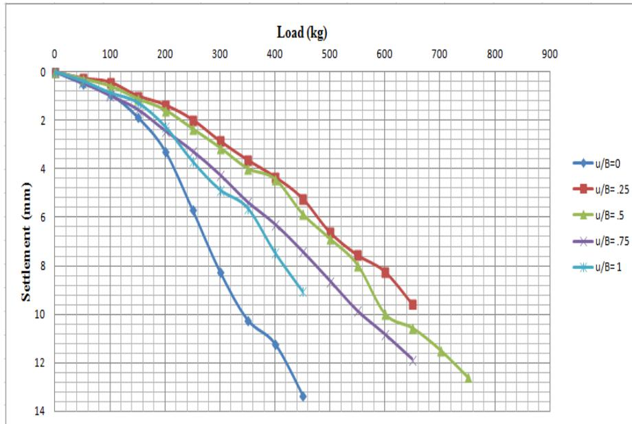
Fig.10. Combined load vs settlement at various  $u/B$  ratio
