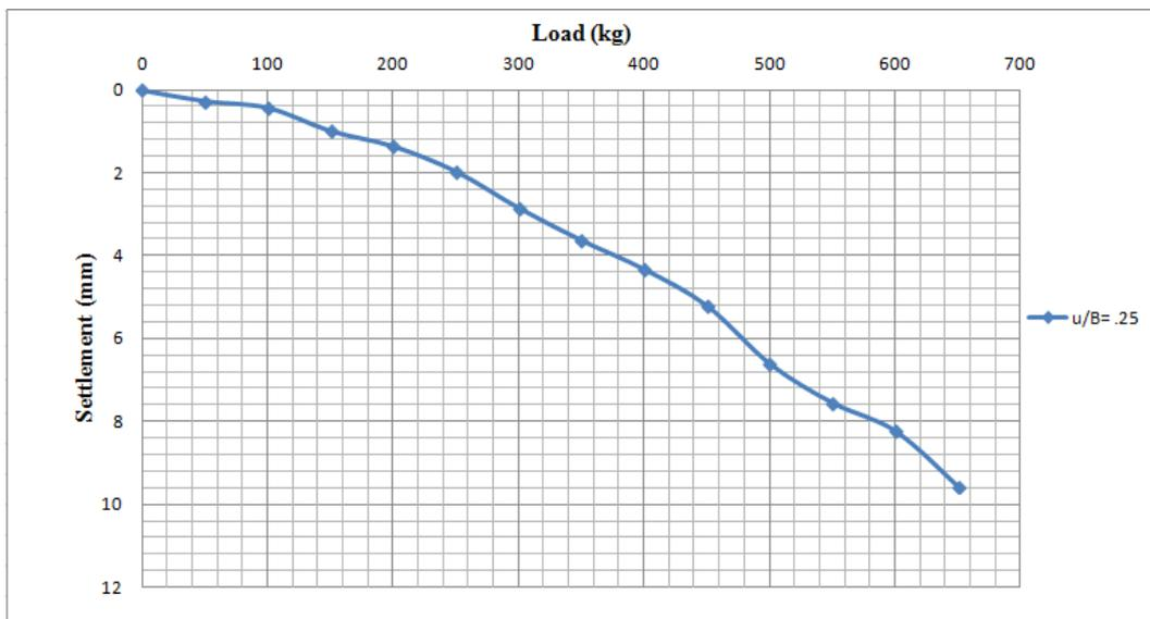
Fig.6. Load vs settlement curve for reinforced sand bed having  $u/B=0.25$
