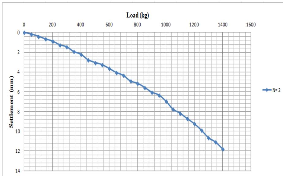
**Fig.12.** Load vs settlement curve for two layers of WGF reinforcement
