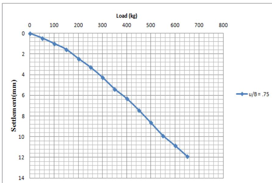
**Fig.8.** Load vs settlement curve for reinforced sand bed having  $u/B=0.75$
