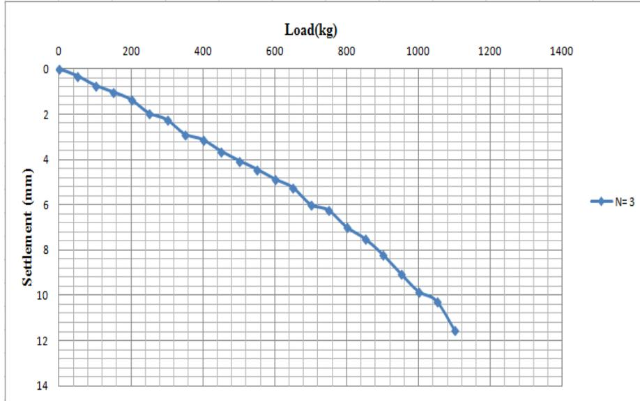
Fig.13. Load vs settlement curve for three layers of WGF reinforcement
