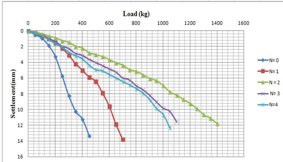
**Fig.15.** Combined load vs settlement for multiple layer reinforcement
