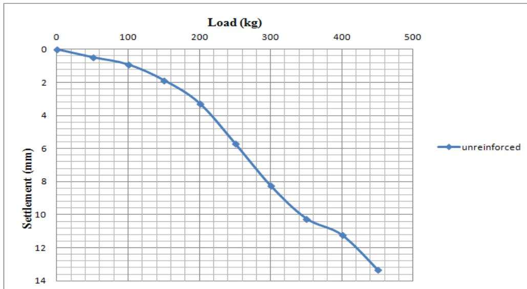
Fig.5. Load vs settlement curve for unreinforced sand bed
