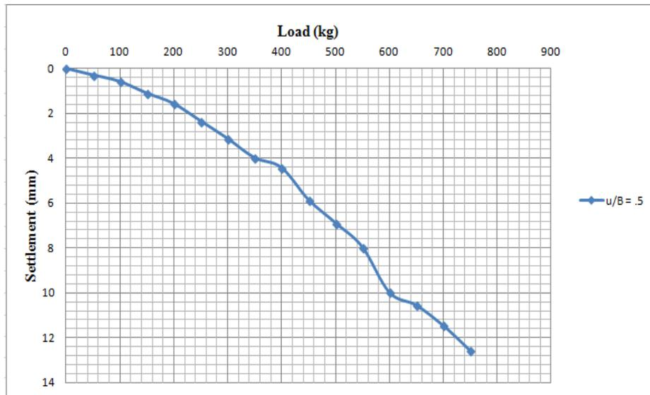
**Fig.7.** Load vs settlement curve for reinforced sand bed having  $u/B=0.5$
