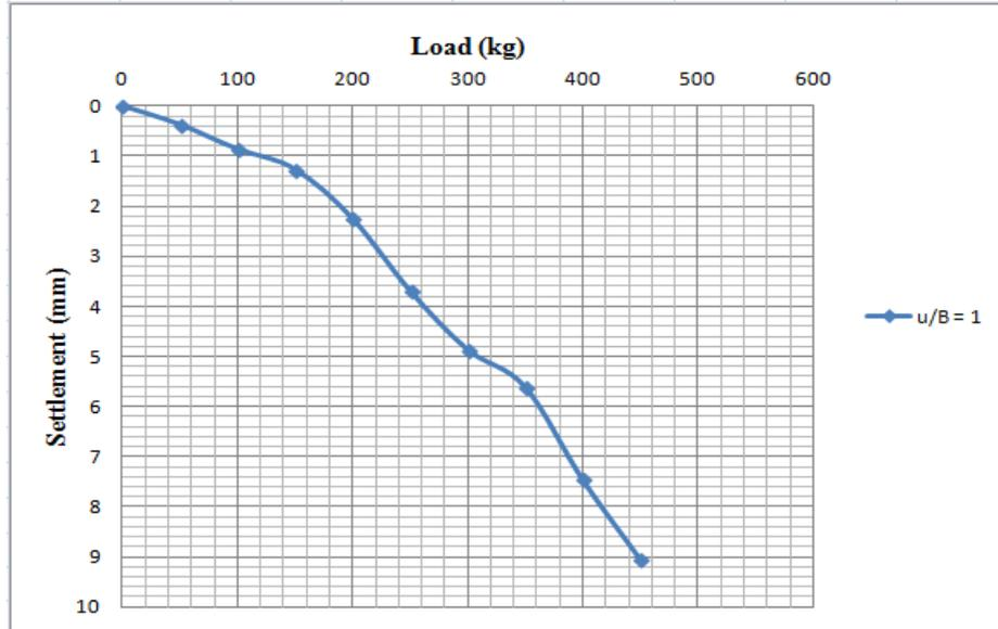
Fig.9. Load vs settlement curve for reinforced sand bed having  $u/B=1.0$
