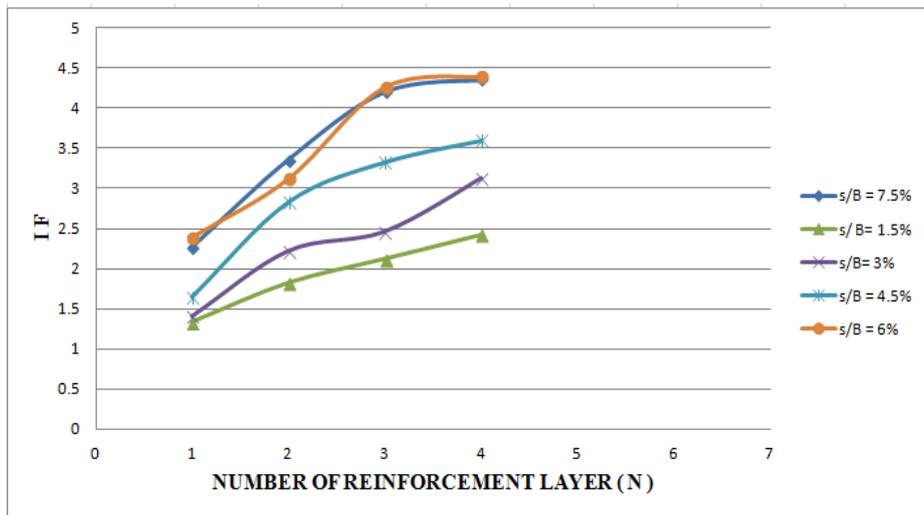
**Fig.16.** Improvement factor vs the number of reinforcement layers at s/B ratios
