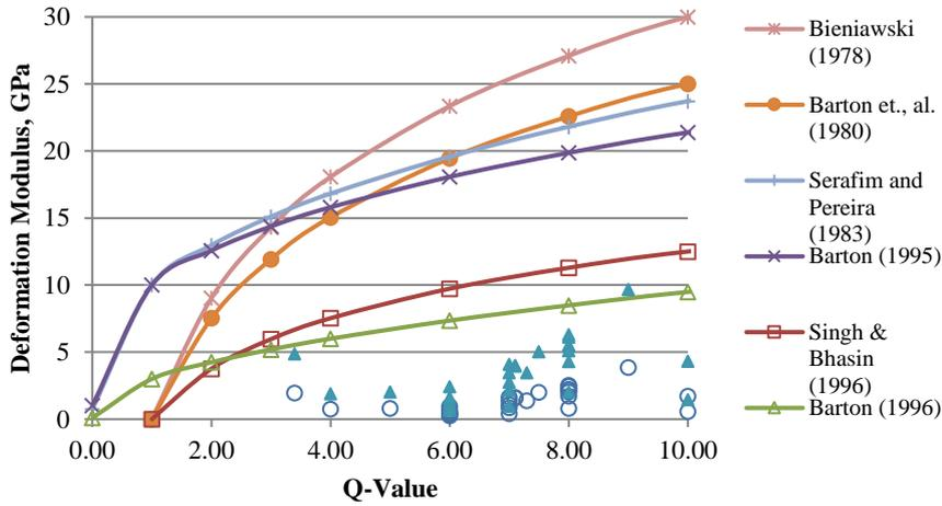
**Fig.1.** In-situ plate load test data along with envelope of empirical equations
