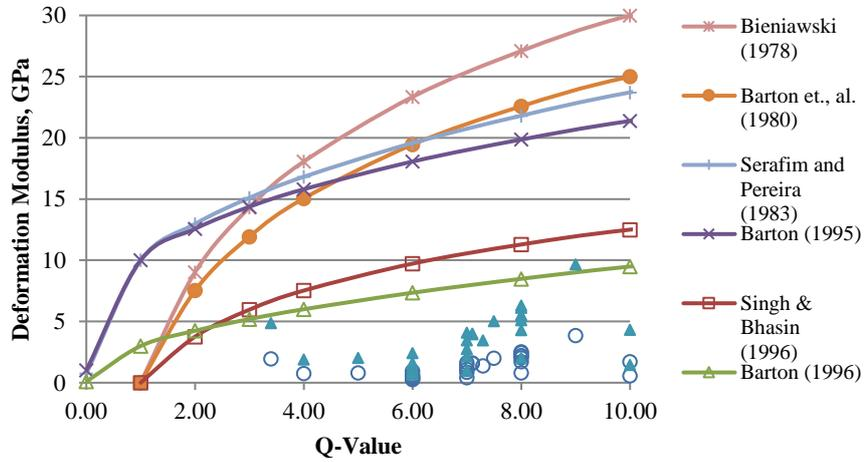
**Fig.1.** In-situ plate load test data along with envelope of empirical equations
