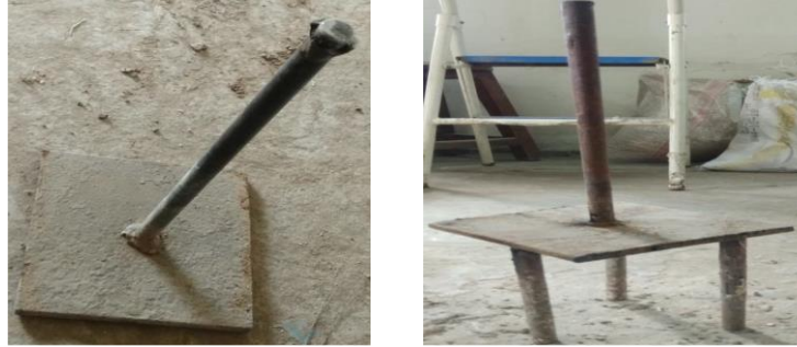
Fig.3. Fabricated micropile system includes a footing plate with micropile (Left) and footing plate with three micropiles (Right)
