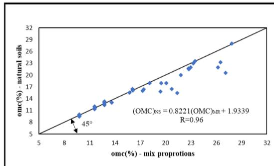
**Fig. 19.** variation of OMC(%) of natural soils with OMC(%) of mix proportions of standard Proctor test.
