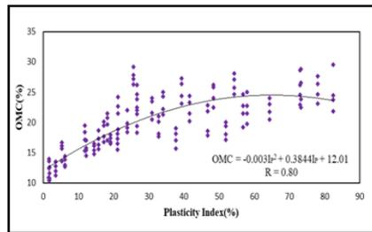
**Fig. 8.** variation of OMC(%) with Plasticity index, I<sub>p</sub> (%).
