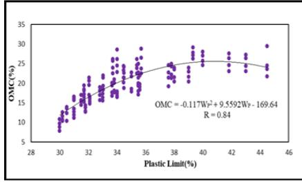
**Fig. 6.** variation of OMC (%) with plastic limit, W<sub>P</sub> (%).
