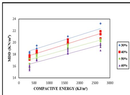
**Fig.12.** variation of MDD(KN/m<sup>3</sup>) with compactive energy.
