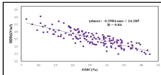
**Fig. 11.** variation of MDD,  $\gamma_{d\max}$ (KN/m<sup>3</sup>) with OMC (%) different compactive energy levels.
