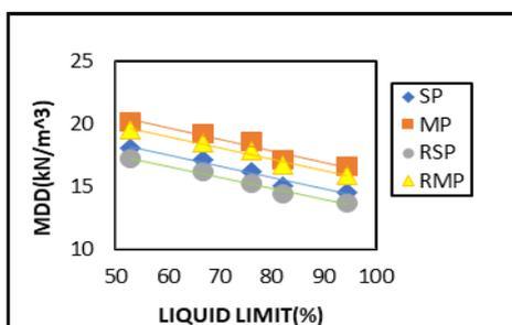
**Fig. 1.** variations of liquid limit,  $W_L$ (%) with MDD ( $KN/m^3$ ) for constant bentonite
