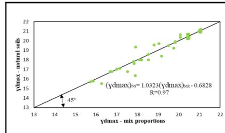
**Fig.18.** variation of MDD (KN/m<sup>3</sup>) of natural soils with MDD(KN/m<sup>3</sup>) of mix proportions of reduced standard Proctor test.
