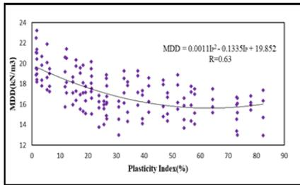
**Fig. 7.** variation of MDD(kN/m<sup>3</sup>) with index, I<sub>p</sub> (%).
