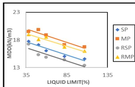
**Fig. 2.** variation of liquid limit,  $W_L$ (%) with MDD ( $KN/m^3$ ) for constant kaolinite
