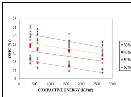
**Fig. 13.** variation of OMC (%) with compactive energy.
