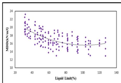
**Fig. 3.** variation of MDD (KN/m<sup>3</sup>) with Liquid limit, W<sub>L</sub> (%).
