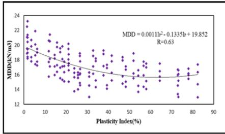
**Fig. 5.** variation of MDD(KN/m<sup>3</sup>) with plastic limit, W<sub>P</sub> (%).
