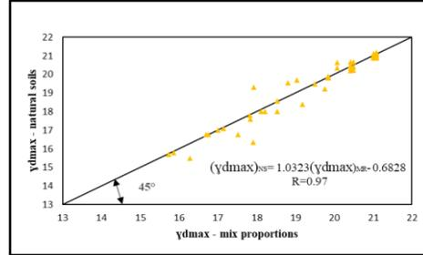
**Fig.16.** variation of MDD(KN/m<sup>3</sup>) of natural soils with MDD (KN/m<sup>3</sup>) of mix proportions of reduce modified Proctor test.
