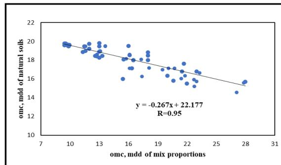
**Fig.20.** variation of OMC(%), MDD(KN/m<sup>3</sup>) of natural soils with OMC(%), MDD(KN/m<sup>3</sup>) of mix proportion of standard Proctor test
