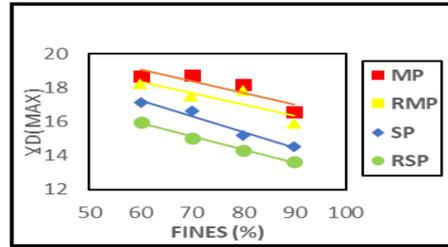
**Fig.10.**variation of MDD,  $\gamma_{d\max}$ (KN/m<sup>3</sup>) with percent fines, PF(%) for constant bentonite, kaolinite.
