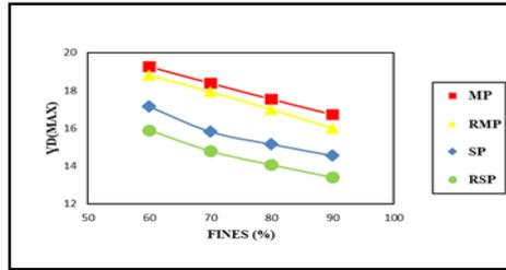
**Fig. 9** variation of MDD,  $\gamma_{d\max}$ (KN/m<sup>3</sup>) with percent fines, PF(%) for constant bentonite, kaolinite.
