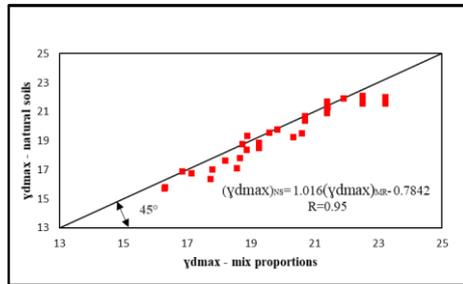
**Fig. 15.** variation of MDD(KN/m<sup>3</sup>) of natural soils with MDD (KN/m<sup>3</sup>) of mix proportions of modified Proctor test.
