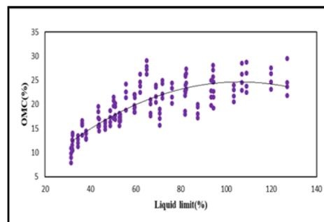
**Fig. 4.** variation of OMC (%) with Liquid limit, W<sub>L</sub> (%).
