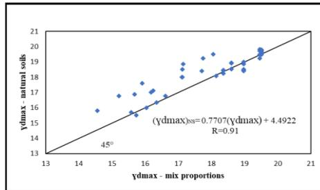
**Fig. 17.** variation of MDD (KN/m<sup>3</sup>) of natural soils with MDD(KN/m<sup>3</sup>) of mix proportions of standard Proctor test.
