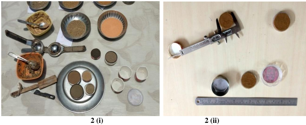
Fig.2. (i and ii). Dish Method for Determination of Volumetric Shrinkage (%) of Soils.
