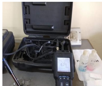
Fig.2 Determination of pH With pH Meter
