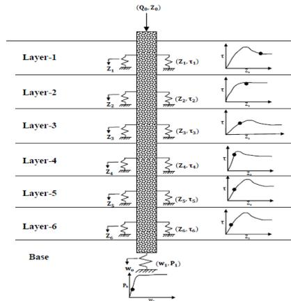
Fig. 1 Load-transfer concept for a vertical compressible pile
