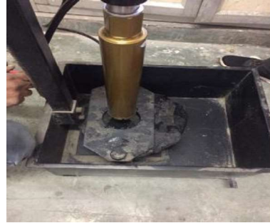
Fig. 2. Core Drilling Specimen
