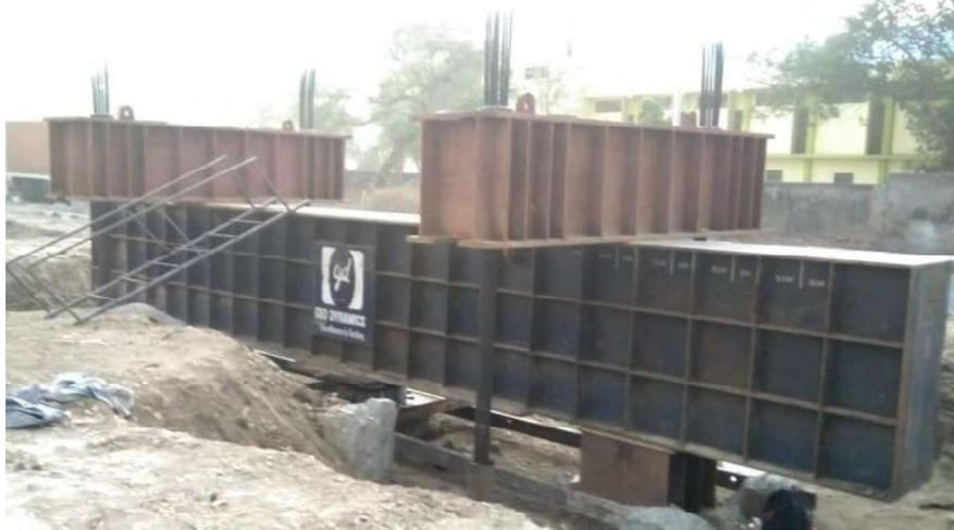
**Fig. 2.** Vertical Load Test in Progress at a site in Nagpur
