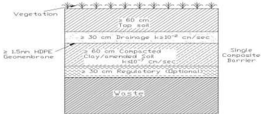
Fig. 1. Cover system for Hazardous waste landfill, CPCB, 2001
