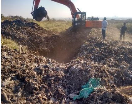
Fig. 1. Collection of samples of aged MSW from a pit at dump site
