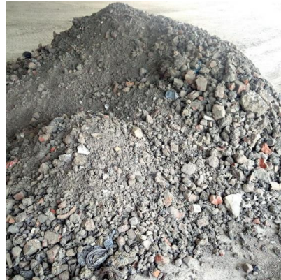
Fig.2. Stock Pile of Bottom ash
