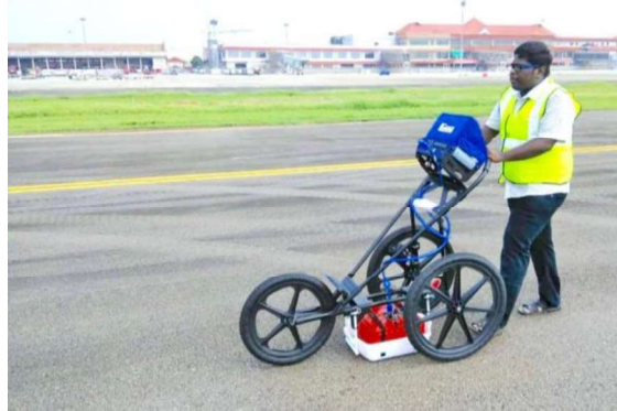
Fig.1. GPR Run in the Runway Lane
