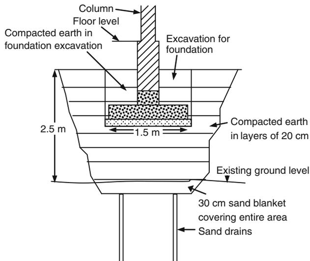
**Fig. 29** Schematic diagram of the proposed scheme
