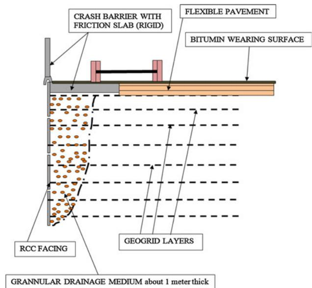
Fig. 9 Schematic diagram of RE wall
