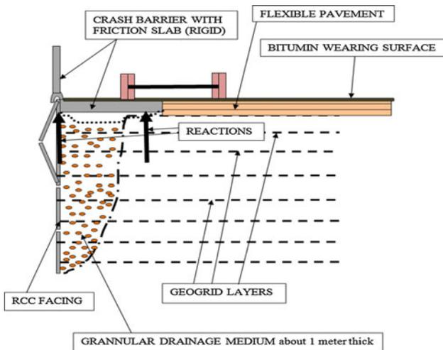
Fig. 10 Schematic diagram of failure condition
