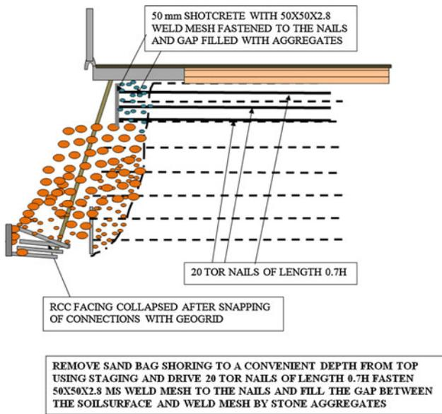
Fig. 14 Incremental removal of sand bag shoring and soil nailing
