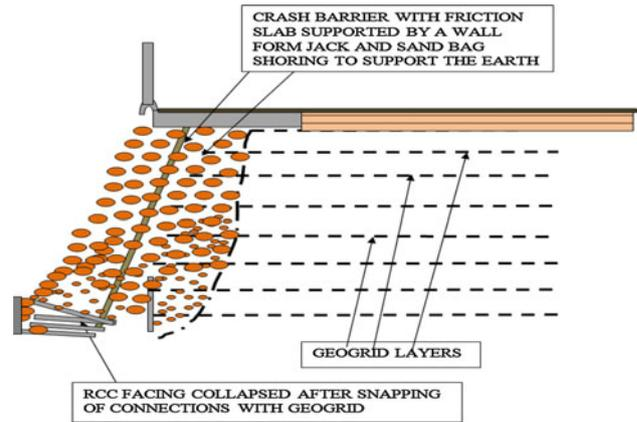
Fig. 11 Schematic diagram of sand bag shoring
