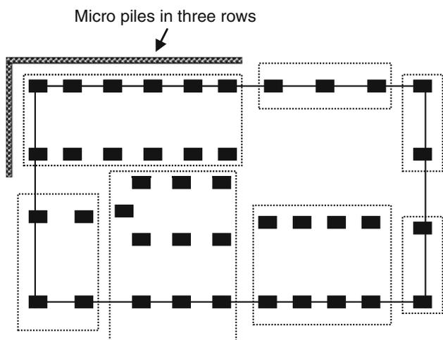
**Fig. 4** Scheme of remedial measures
