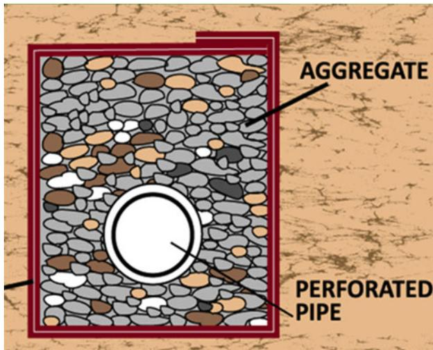
Fig. 45 Typical French drain
