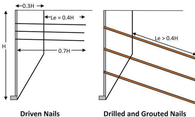
**Fig. 92** Design principle of driven and grouted nails
