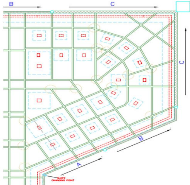
**Fig. 44** Plan of the under slab drainage system
