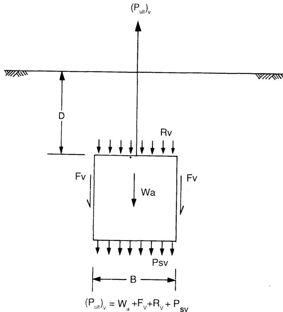
FIGURE 54. Forces Contributing to Breakout Capacity
