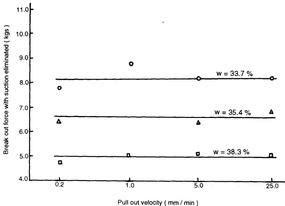
FIGURE 56. Breakout Force with Suction Eliminated not Influenced By Pull Out Velocity After Baba et. al. (1989)
