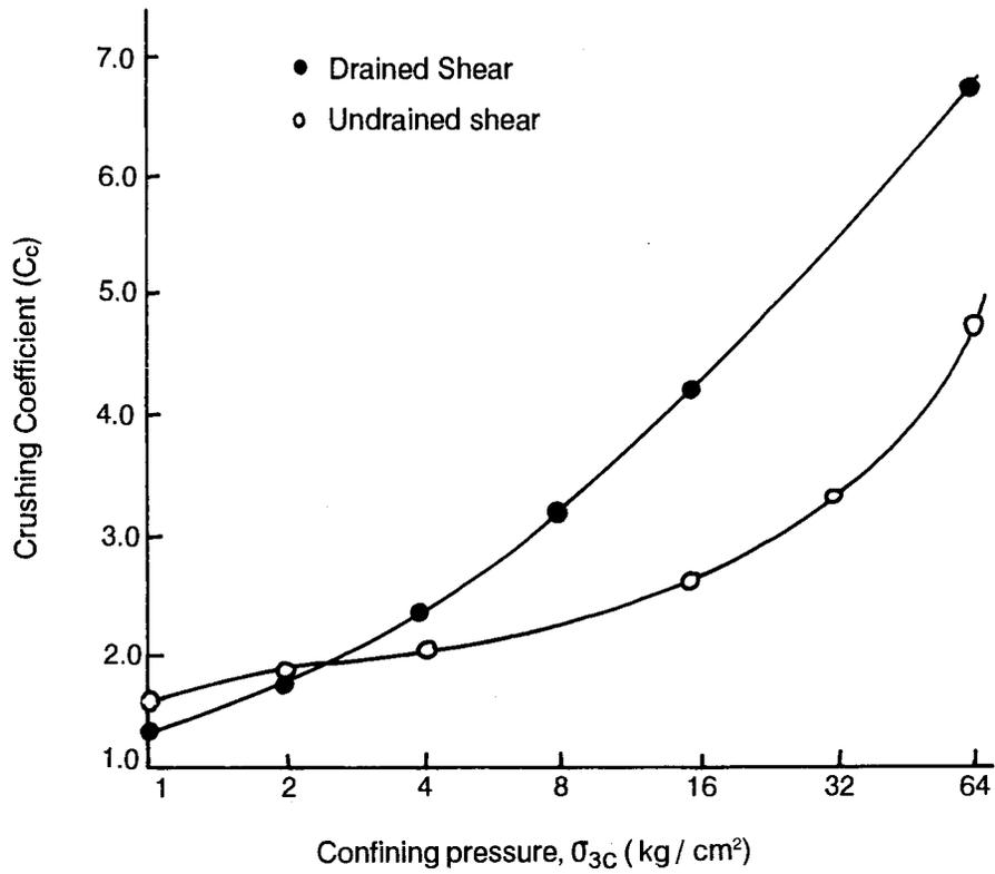
FIGURE 22. Variation of Crushing Coefficient with Confining Pressure for Sand A—After Datta et. al. (1979)
