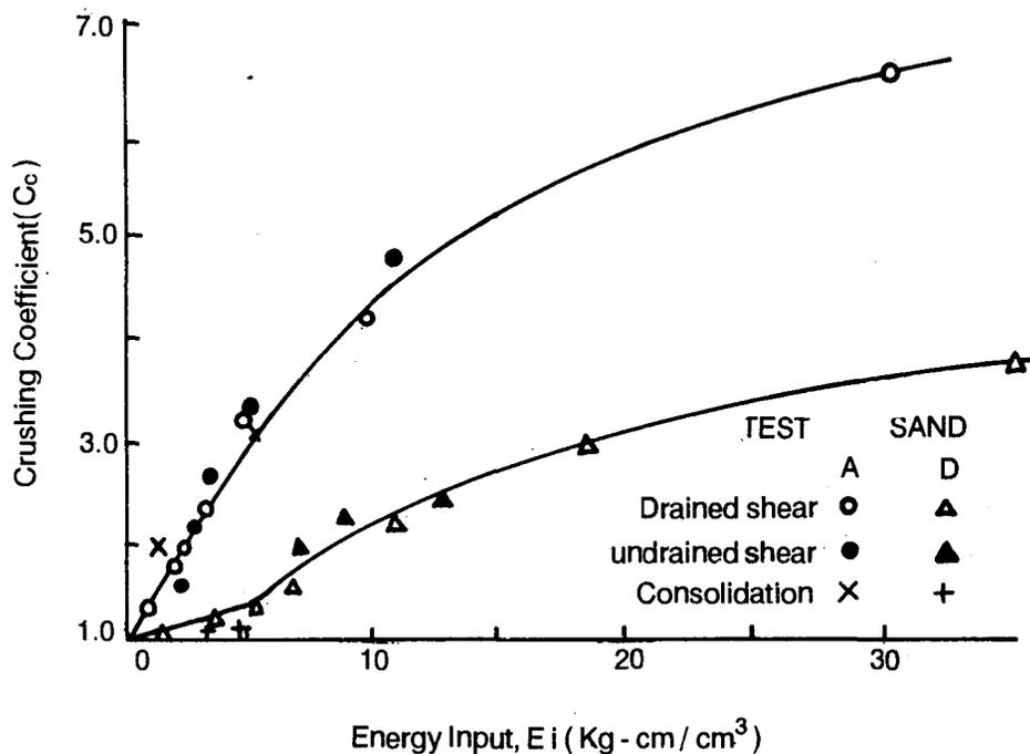
FIGURE 26. Variation of Crushing Coefficient with Energy Input—After Datta et. al. (1980a)
