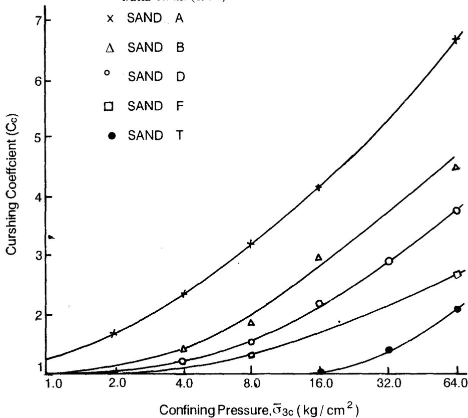
FIGURE 17. Effect of Confining Pressure on Post-Shear Crushing Coefficient in Drained Tests--After Datta et. al. (1980).
