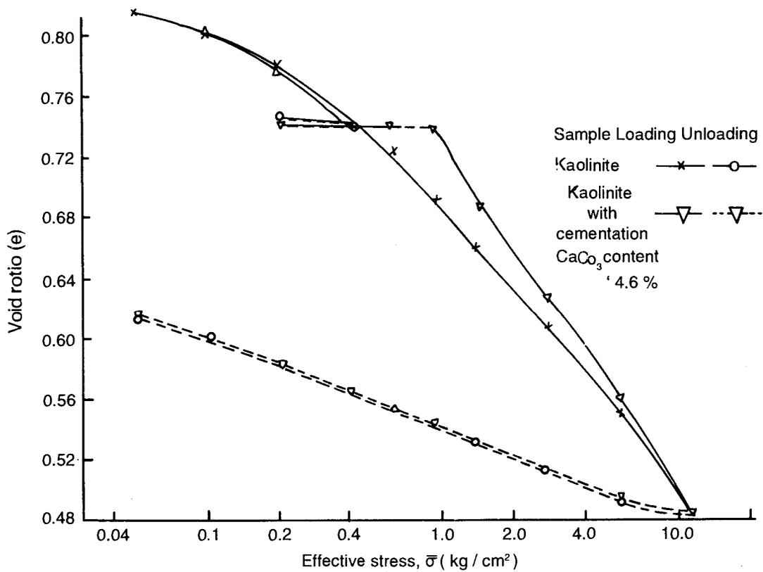
FIGURE 34. One-Dimensional Consolidation Curves for Kaolinite with and without cementation—After Nambiar (1982)
