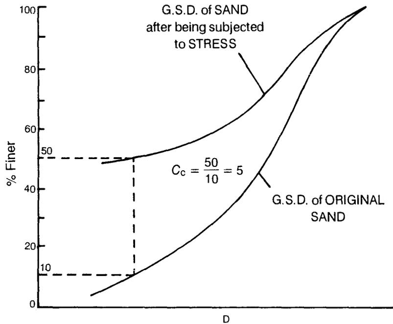
FIGURE.16 Method of Determining Crushing Coefficient - After Datta et. al. (1980)
