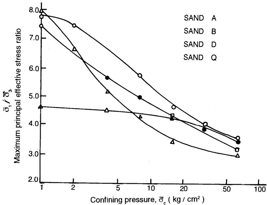
**FIGURE 21. Influence of Confining Pressure on the Maximum Principal Effective Stress Ratio—After Datta et. al. (1980)**
