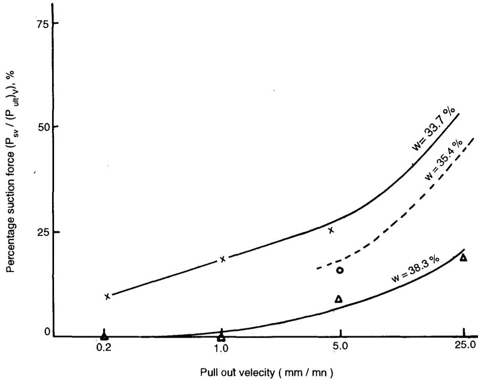
FIGURE 57. Increase in Suction Force with Increase in Pull out Velocity--After Baba *et. al.* (1989)
