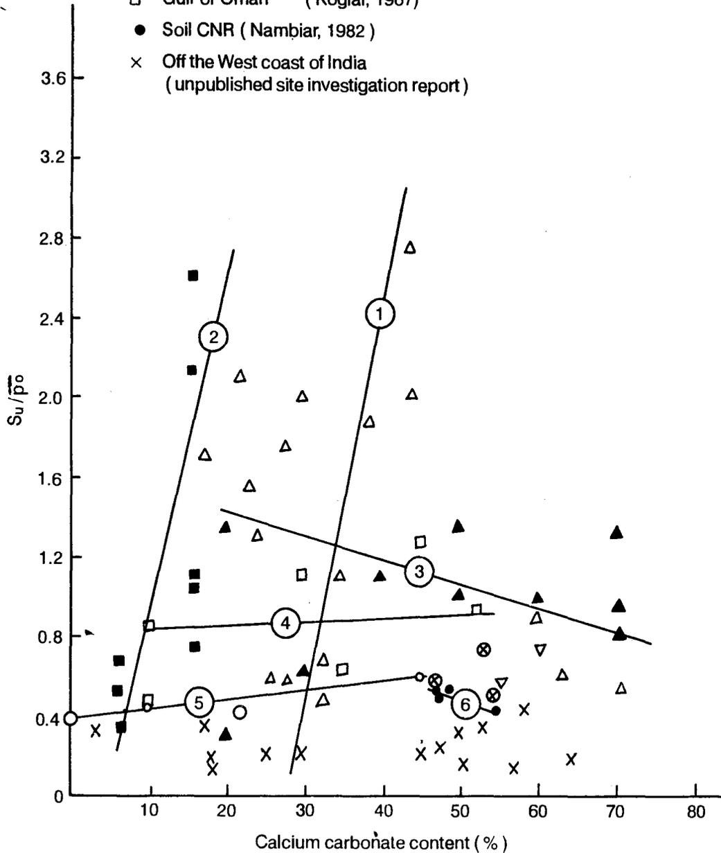
FIGURE 31. Variation of  $S_u/p_o$  with Calcium Carbonate Content—After Nambiar (1982)
