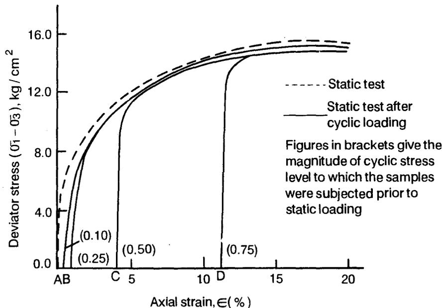
FIGURE 30. Static Stress-Strain Behaviour After Cyclic Loading—After Datta et. al. (1980b)
