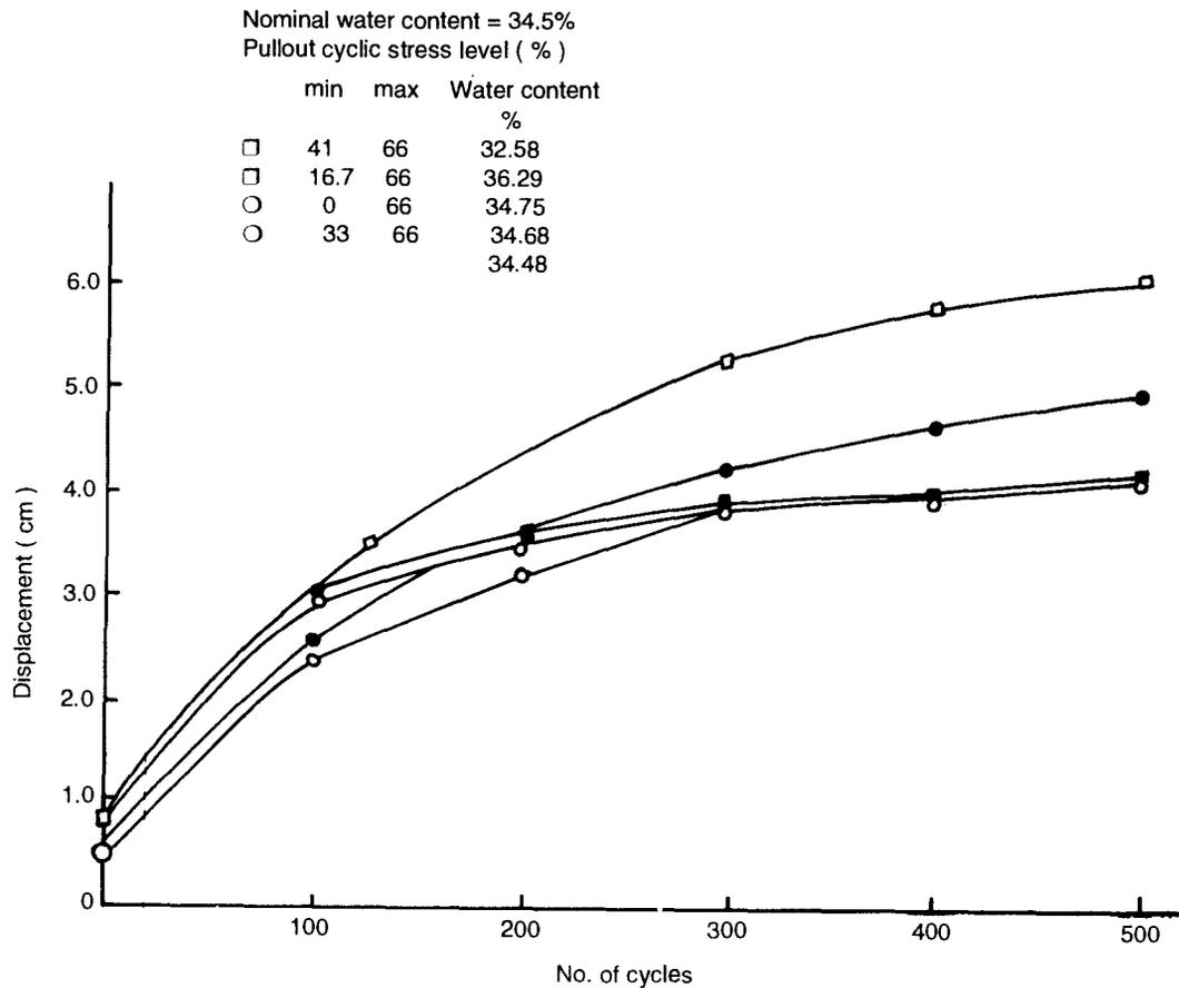
FIGURE 59. Movement of Plate Anchors with Number of Cycles for a Maximum Cyclic Stress Level of 66% After Datta *et. al* (1990)
