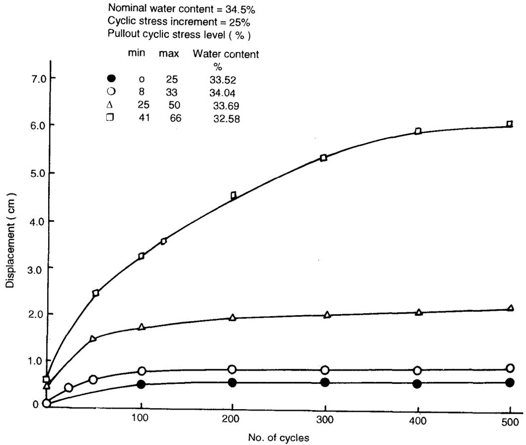
FIGURE 58. Movement of Plate Anchors with Number of Cycles for a Constant Cyclic Stress Increment--After Datta *et. al.* (1990)
