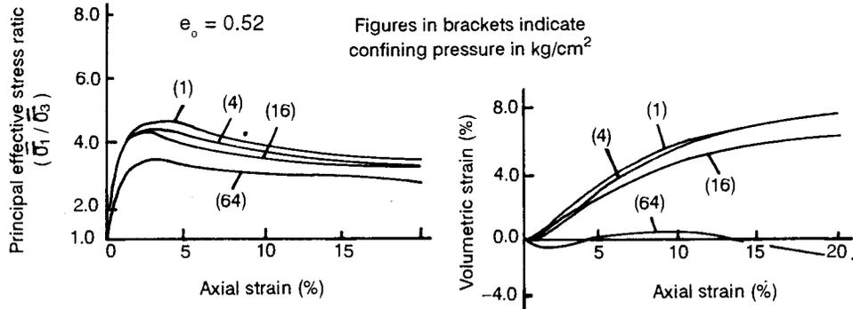
**FIGURE 20. Stress-Strain-Volume Change Behaviour for Sand T—After Datta et. al. (1980)**
