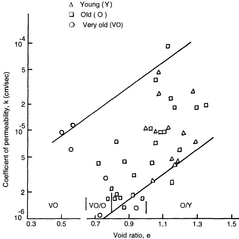
FIGURE 44. Variation of Coefficient of Permeability with Void Ratio for Rocks of Group-II--After Deshmukh (1983)
