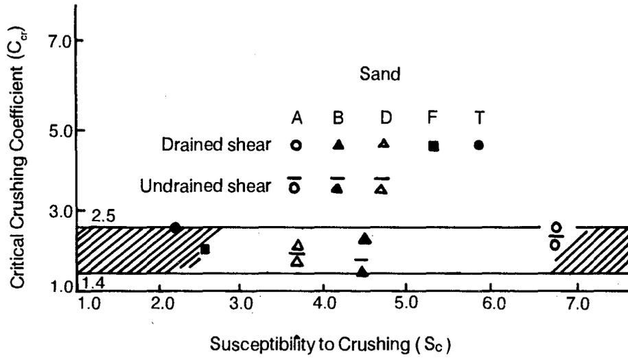
FIGURE 27. Relation Between Critical Crushing Coefficient and Susceptibility to Crushing—After Datta et. al. (1980a)
