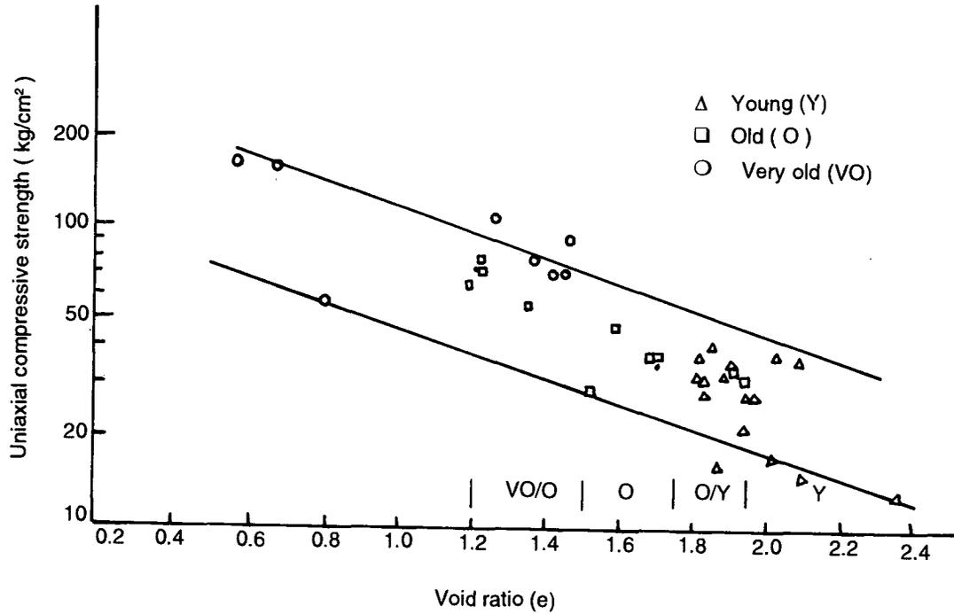
FIGURE 46. Variation of Uniaxial Compressive Strength with Void Ratio for Rocks of Group-I--After Deshmukh (1983)
