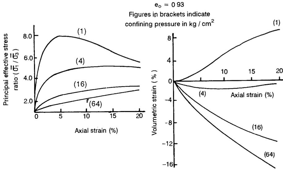
**FIGURE 19. Stress-Strain-Volume Change Behaviour for Sand A—After Datta et. al. (1980)**
