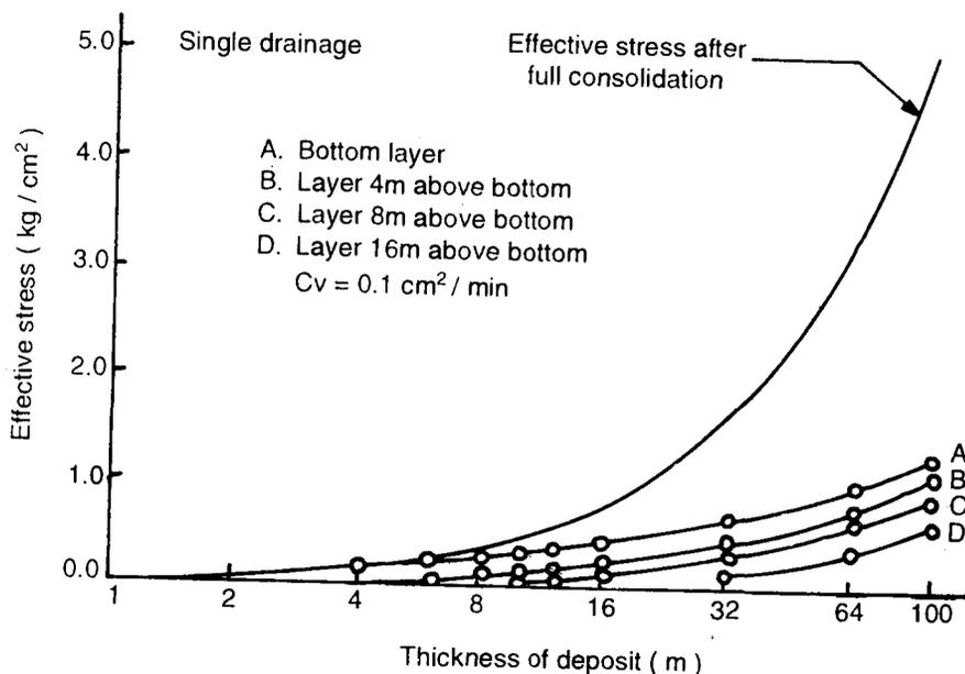
FIGURE 52. Variation of Effective Stress with Time at Different Locations--After Datta *et. al.* (1983)
