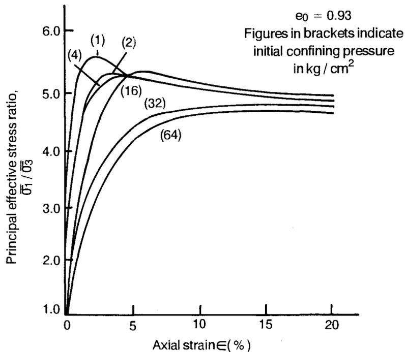
FIGURE 24. Variation of Principal Effective Stress Ratio with Strain for sand A—After Datta et. al. (1979)
