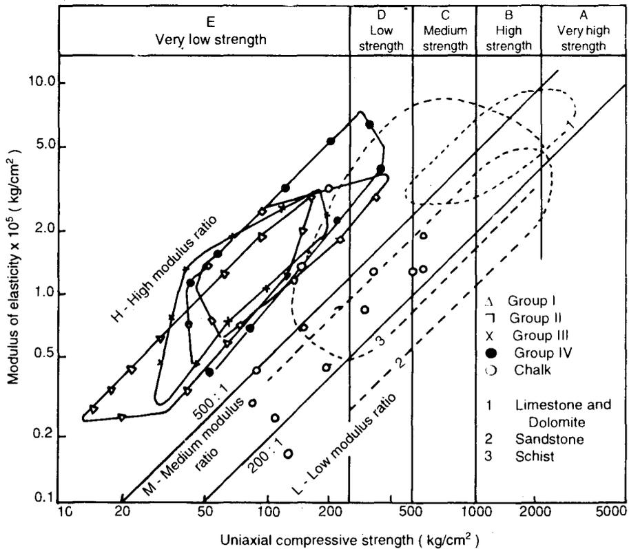
FIGURE 50. Relationship of Uniaxial Compressive Strength and Modulus of Elasticity--After Deshmukh (1983)
