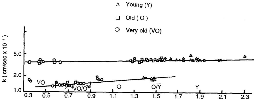
FIGURE 45. Variation of Coefficient of Permeability with Void Ratio for Rocks of Group-IV After Deshmukh (1983)
