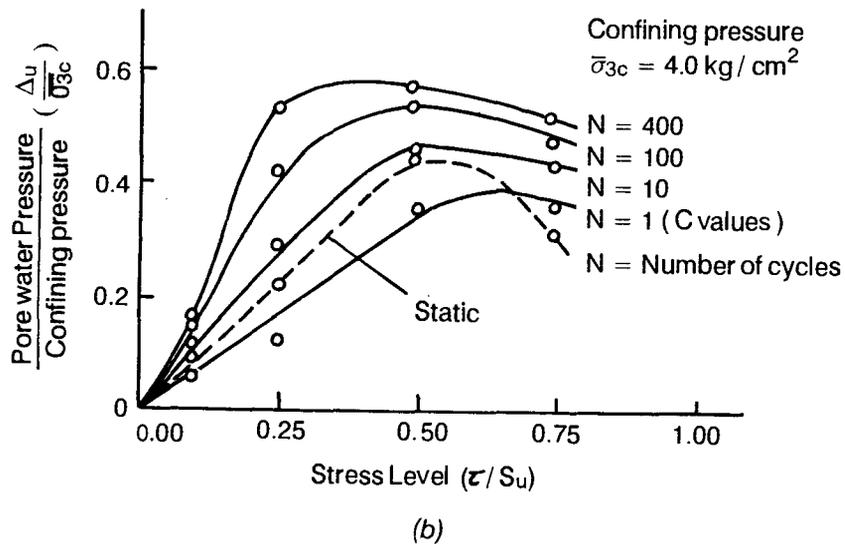
FIGURE 28. Variation of Induced Pore Water Pressure with Stress Level—After Datta et. al. (1980b)
