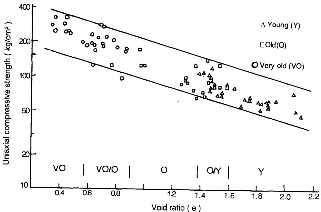
FIGURE 47. Variation of Uniaxial Compressive Strength with Void Ratio for Rocks of Group IV After Deshmukh (1983)
