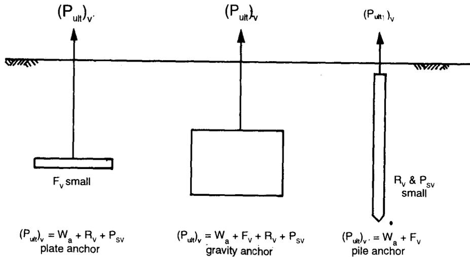
FIGURE 55. Influence of Shape of Anchor on Breakout Capacity
