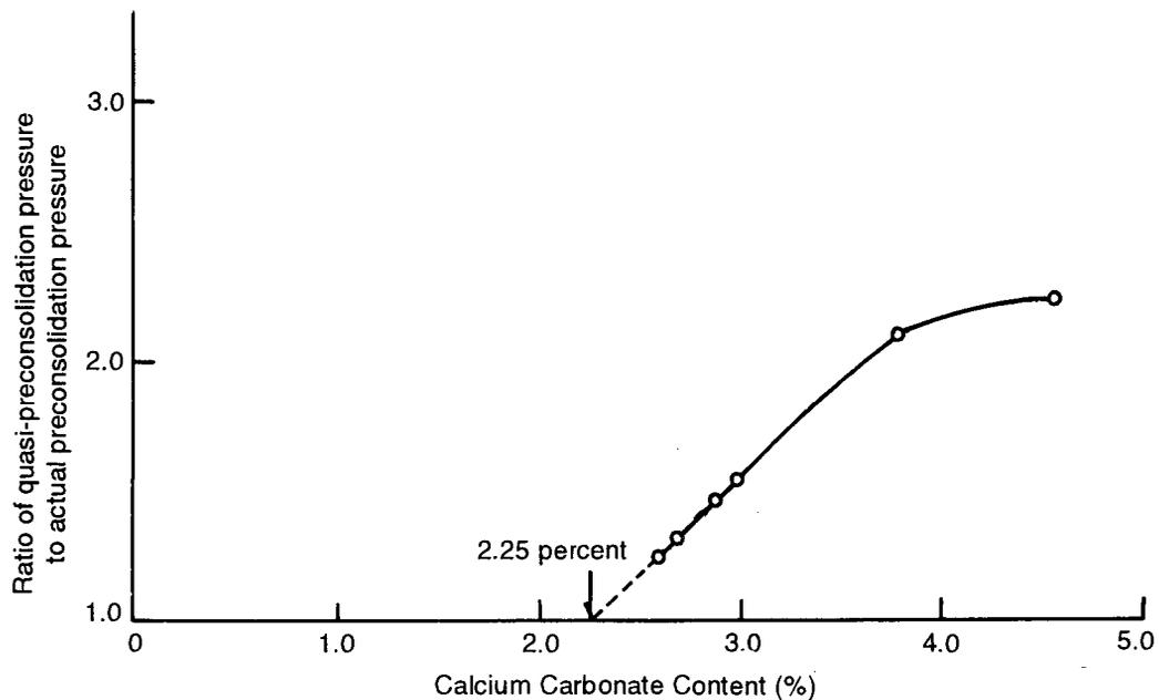
FIGURE 35. Variation of Ratio of Quasi-Preconsolidation Pressure to Actual Preconsolidation Pressure with Calcium Carbonate Content—After Nambiar (1982)
