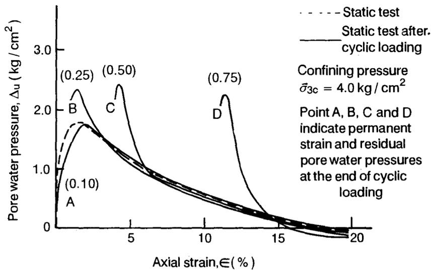
FIGURE 29. Static Pore Water Pressure Strain Behaviour After Cyclic Loading
