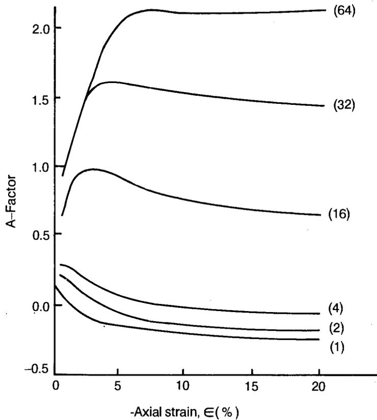
FIGURE 23. Variation of A-Factor with Strain for Sand A—After Datta et. al. (1979)
