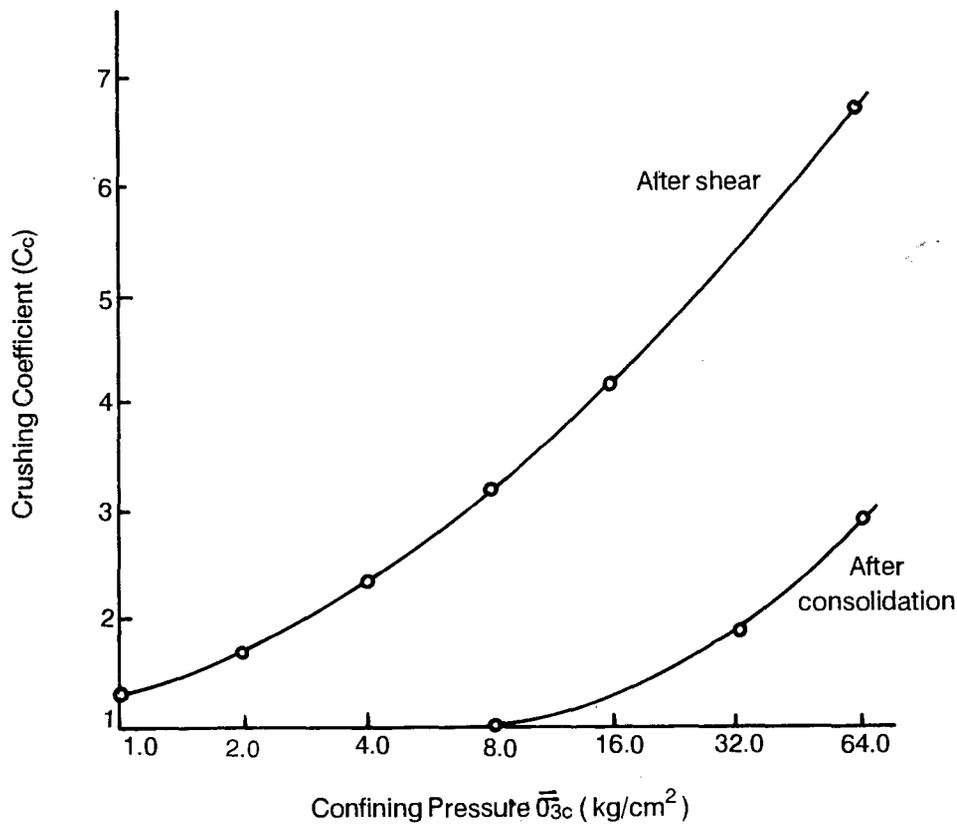
FIGURE 18. Effect of confining Pressure on Crushing Coefficient for Sand A After Consolidation and After Drained Shear—After Datta et. al. (1980)
