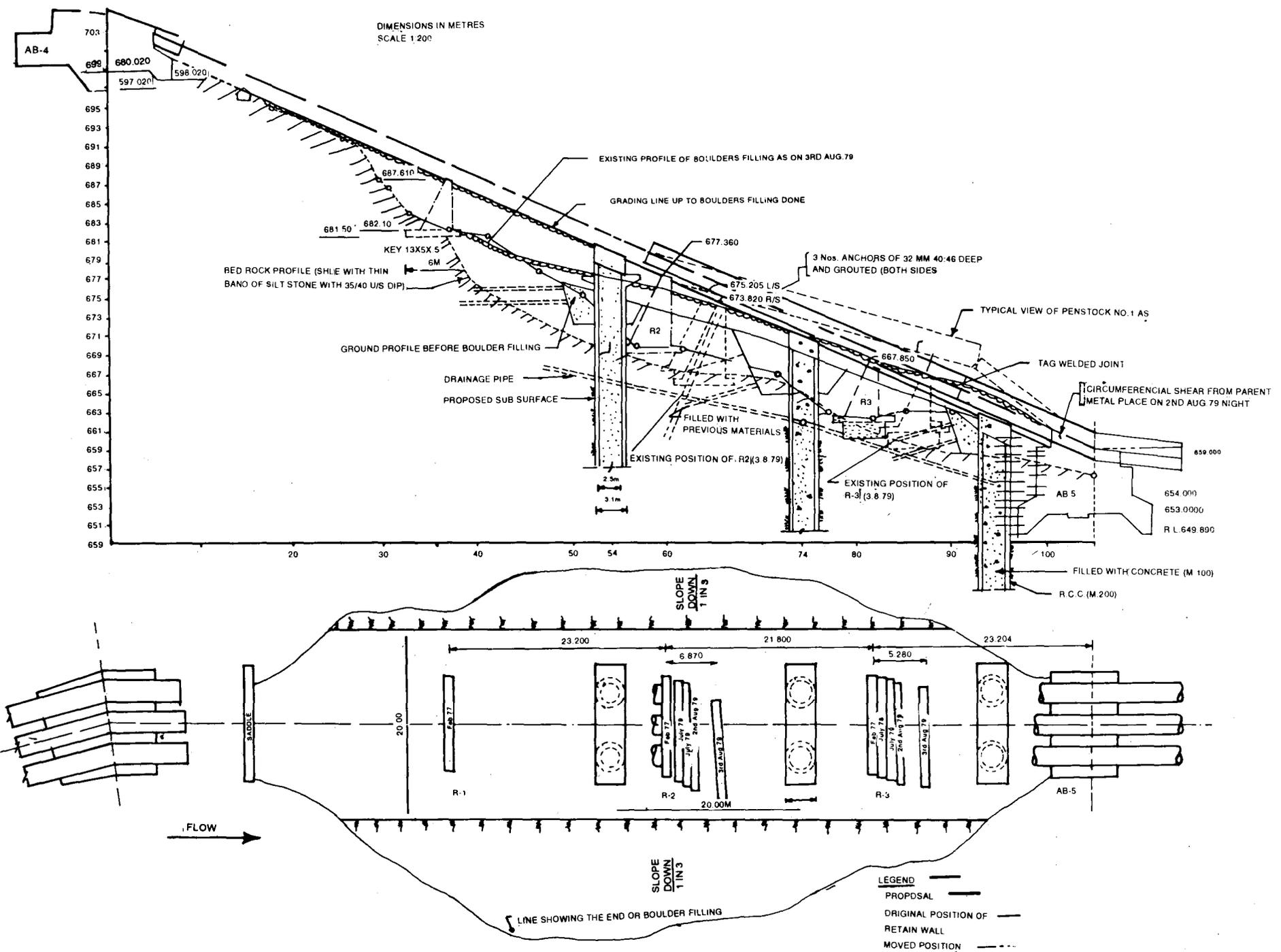
**FIGURE 3 Loktak Hydro-electric Project, Manipur, Plan and longitudinal section of reach anchor block (4-5), showing the details of movement of retaining walls and proposed shafts and drainage**
