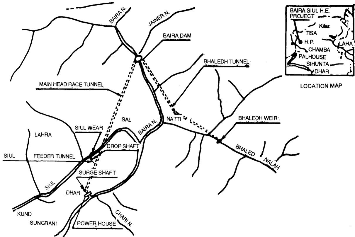
**FIGURE 1 Layout plan of Baira Siul Hydro-electric Project**
