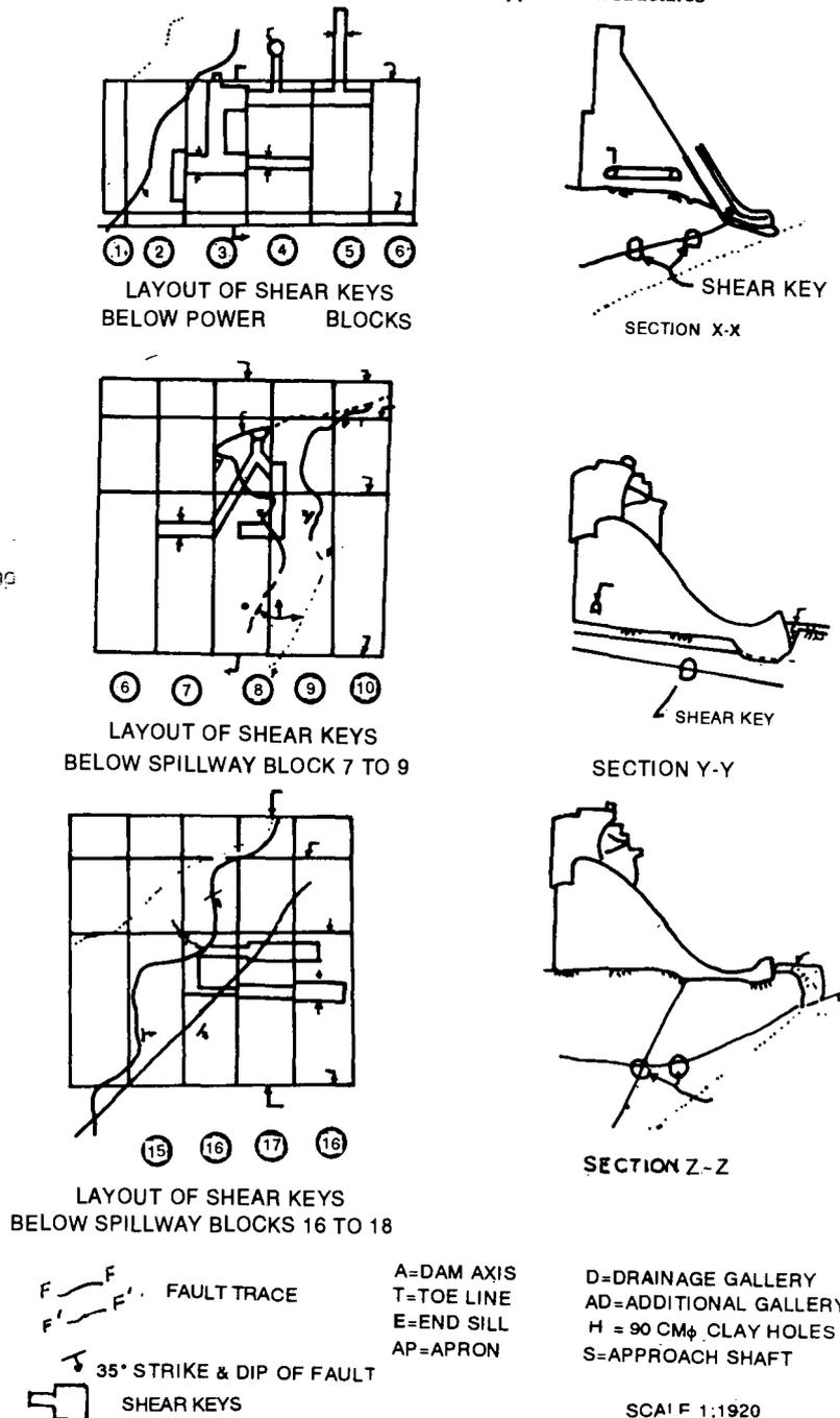
FIGURE 5 Shear keys for treatment of low angle faults below foundations of Kadana dam
