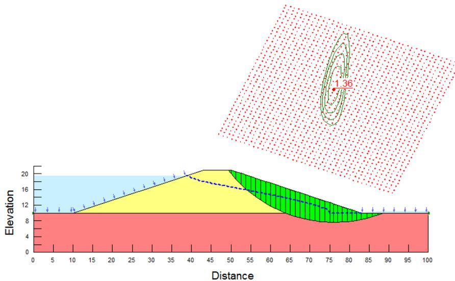
**Fig. 1.** Slope stability analysis of failed section under steady state seepage using GeoStudio
