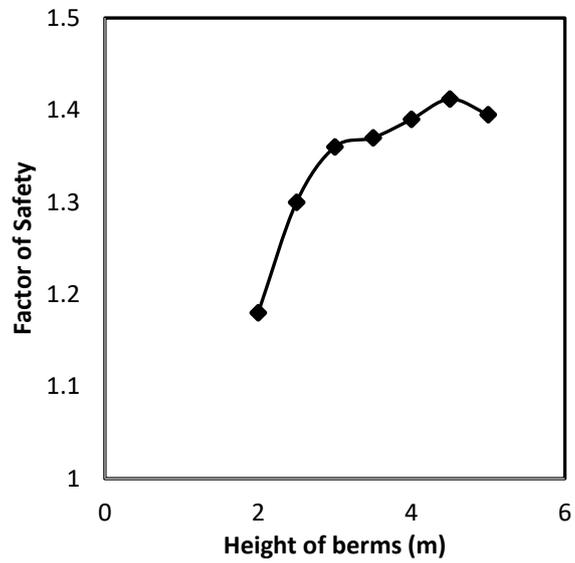
**Fig. 4.** Variation of factor of safety with height of berms
