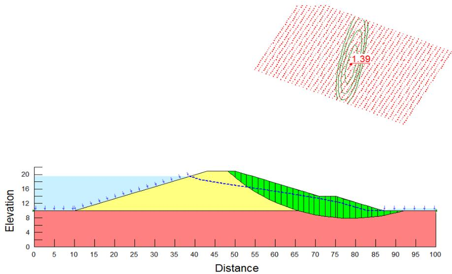
**Fig. 5.** Stability analysis of existing section with berm height 4m
