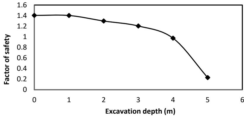
Fig. 2. Variation of factor of safety with excavation depth
