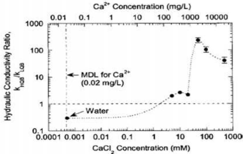
**Fig.1.** Ratio of Hydraulic conductivity of higher quality and lower quality bentonite. [Jae-Myung lee and Charles D. Shackelford.,2005]
